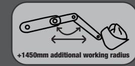
The STOLL telescopic loader concept is equipped with telescopic profiles and an additional swivel axle. The telesopic profiles are made of high-strength and lightweight steel. The profile design is robust and has been tried and tested for many years.
