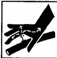
13. Before the first use of the top loading grip and then at least once a year all hoses must be checked by an expert worker for their operational safety and replaced if required. The time of use of the hoses should not exceed six years including a maximum storage time of two years. The replacement hoses and pipings must meet with the implement manufacturer's technical standards.
